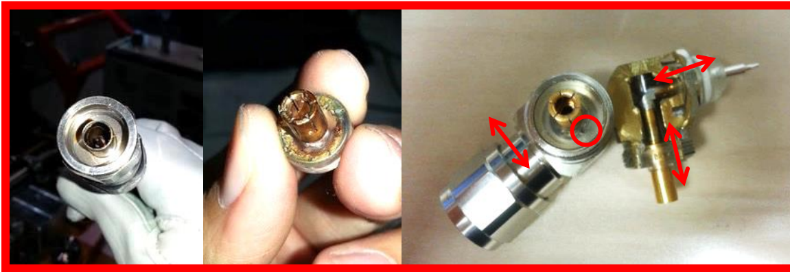
RF glow discharge in closed space of RF connector
