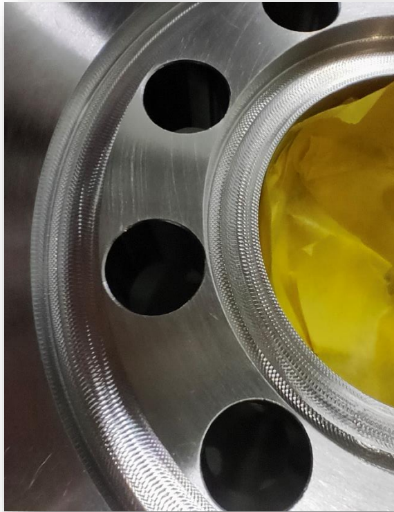
Incorrect sealing surfaces with machining traces
