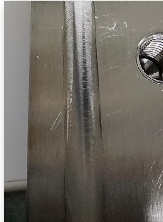
Incorrect sealing surfaces with machining traces
