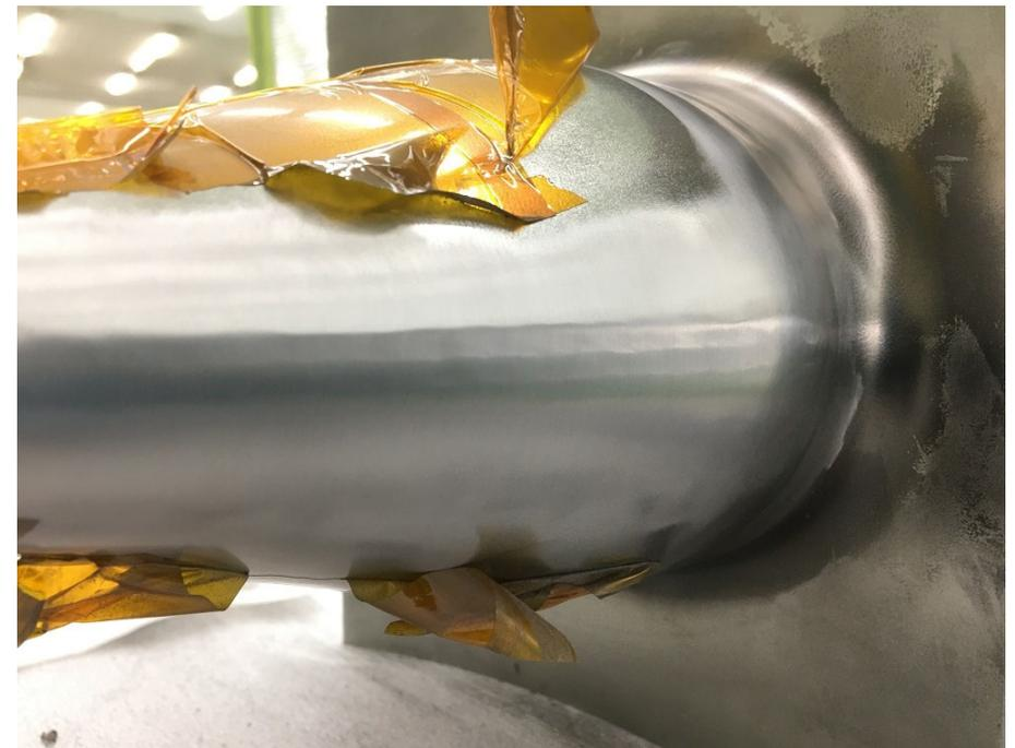
Long radial direction of the elliptical EBW line
