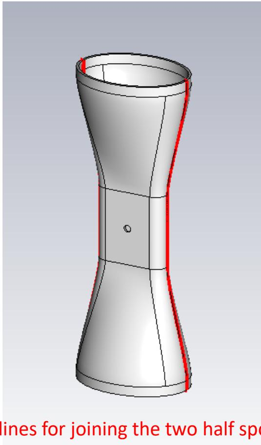
Sloped EBW lines for joining the two half spokes together
