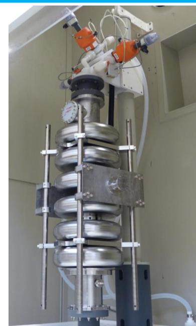
*Treatment of ESS proto M-beta (2016): Standard 'BCP' Chemical polishing*
