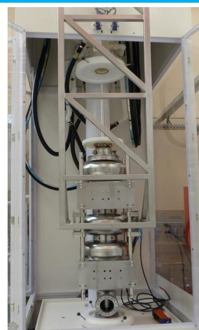
*Treatment of  $\beta=1$  SPL Cavity (2014) (EuCard): Vertical Electropolishing (VEP) with fixed cathode*
