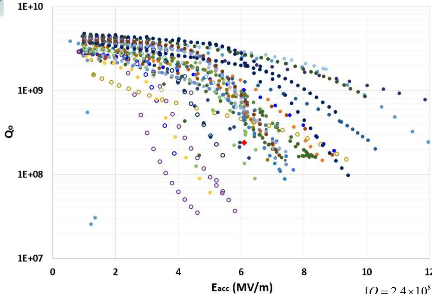
Q slope measurement as a function of accelerating electric field for the quarter-wave resonator (QWR) cavities at 4.2 K. This data shows the failed and passed QWR. The total number of the QWRs is 22 and all of them are passed.
