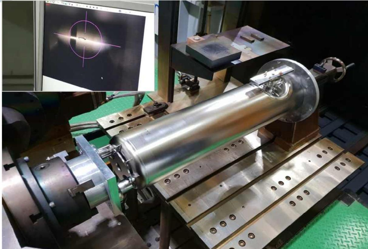
**Electron beam welding**
