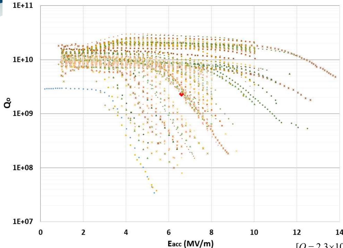
**Q slope measurement as a function of accelerating electric field for the half-wave resonator (HWR) cavities at 2 K. This data shows the failed and passed HWR. The total number of the HWRs is 106 and all of them are passed.**
