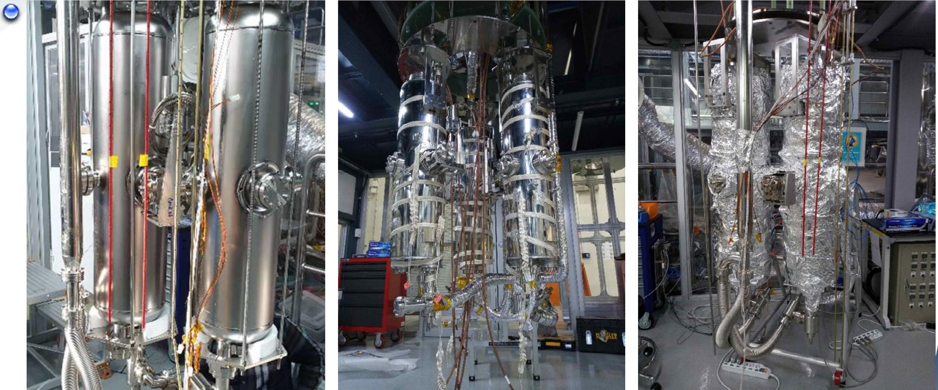
Preparation for the low temperature baking of superconducting cavities
